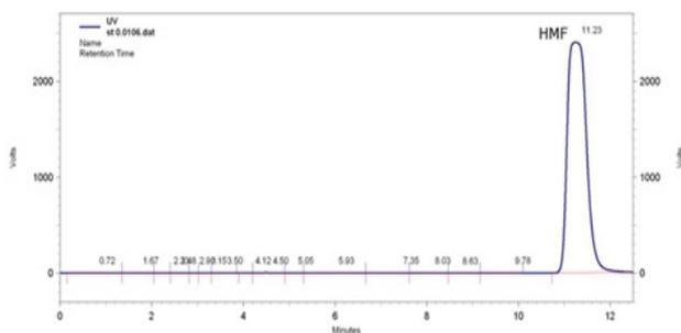
Figure 1. Chromatogram of an HMF standard solution (HMF concentration is 1.06  $\mu$ M). Run time=13 mins and retention time for HMF=11.23 mins
